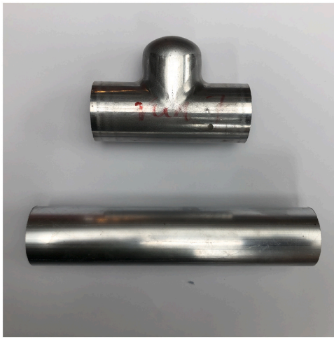
Fig. 10. Illustration of the initial and deformed 6060-O aluminium tubes in hydraulic bulge test with forced end-condition.
