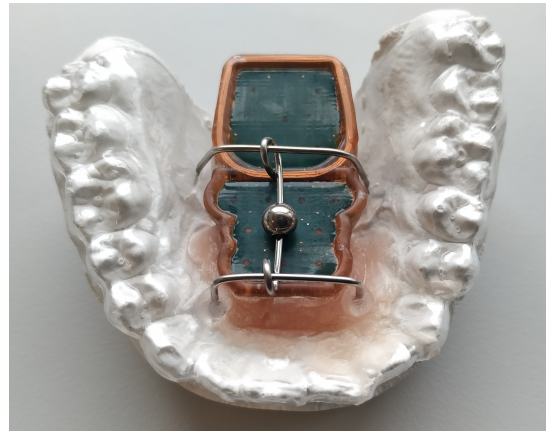
Fig. 3: Noninvasive tongue-computer interface.
