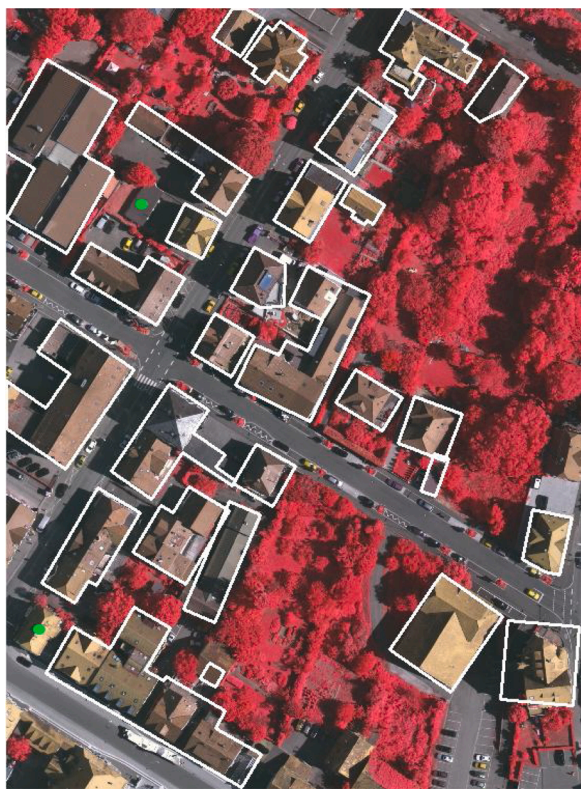
Fig. 5. Enhanced vector data of buildings superimposed onto the DSM-based ortho-image. The green dots mark undetected buildings. Source of ortho-image: ISPRS WG III/4 (2014).
