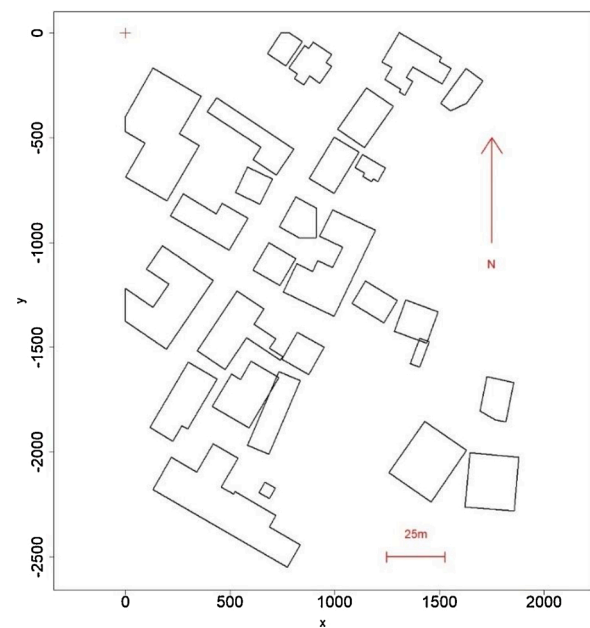
Fig. 4. Vector map derived from the DSM-based ortho-image by the developed method (Vaihingen, Germany, area 7).
