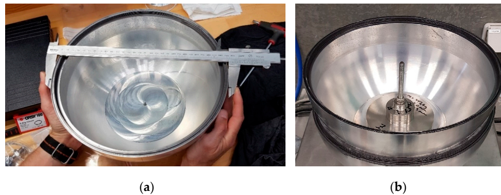
Figure 5. Unballasted hemisphere shell with a diameter of 300 mm (a). Ballasted hemisphere shell with rubber gasket (b).
