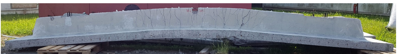
Figure 11. Example of deflected beam after testing.
