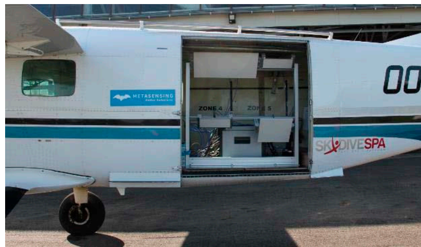
Figure 3. Cessna C208 carrying the SARSense radar setup. The top left and bottom right antennas are for L-band, the bottom left and top right antennas for C-band.
