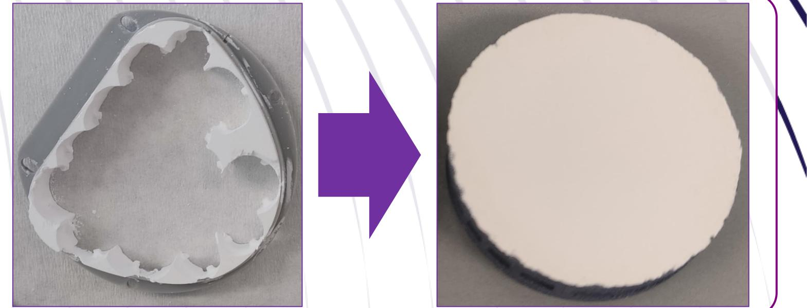
In this project, we use dental zirconia waste in the form of nanopowder to fabricate SiC ceramic membrane with high potential in the **removal** of **oil** residues from **produced water**.
