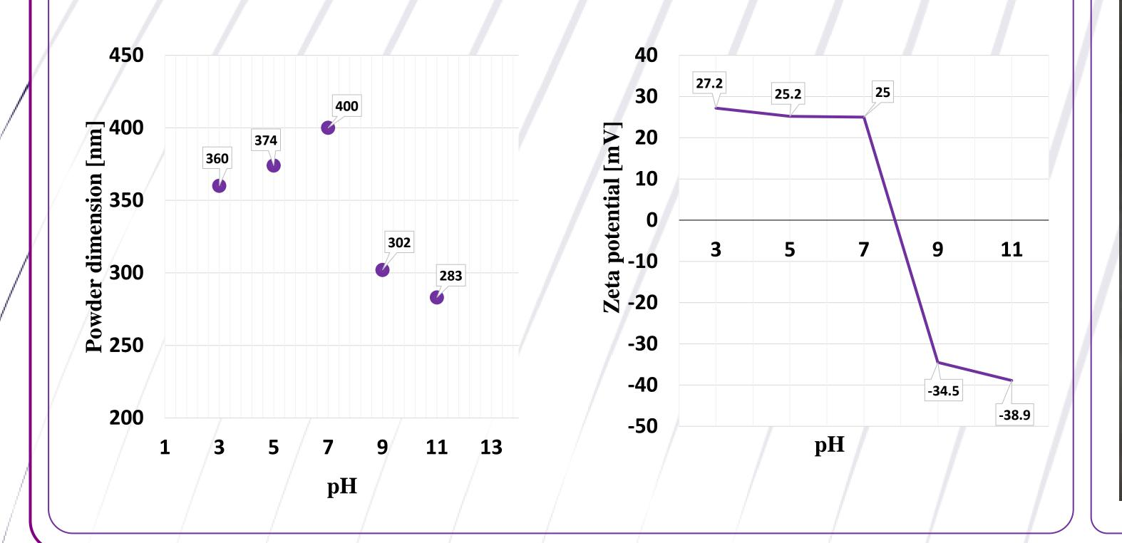
**Ball milling** was performed in order to reduce particles dimensions (DLS measurements).
