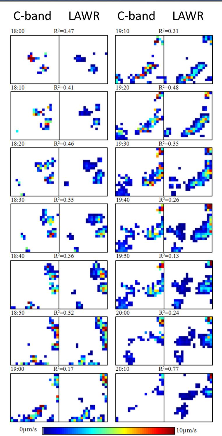
ig. 3 Corresponding precipitation estimates for Cband and LAWR from 06.07.09. The LAWR is averaged in space to fit the 2x2km resolution of the C-band. The area is a 40x40km square with the LAWR in the center *as illustrated in figure 2.*
