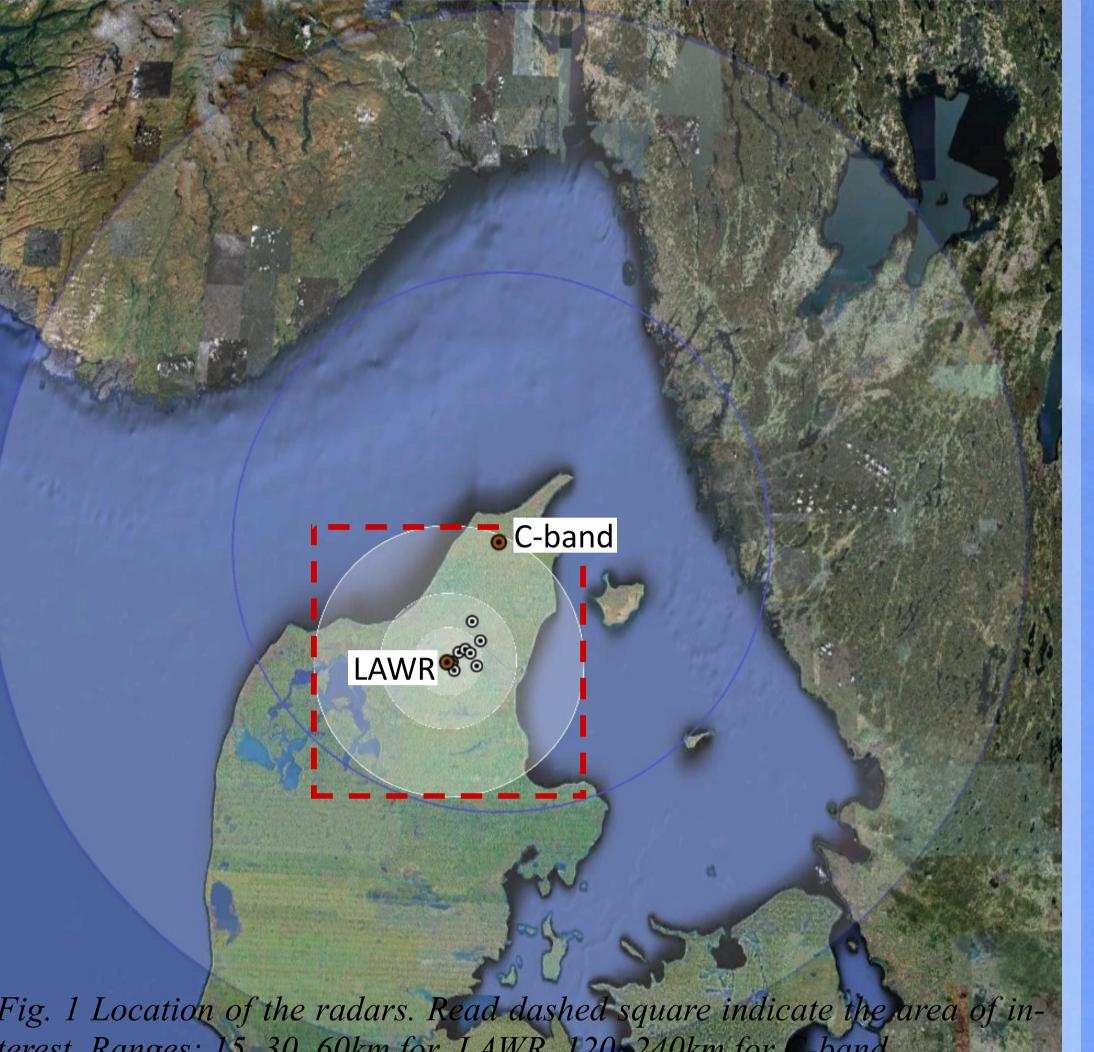
For the comparison, an area of the northern part of Denmark is investigated. The area is covered by both a Local Area Weather Radar (LAWR) and a meteorological C-band radar. The area is instrumented with nine tipping bucket rain gauges.
