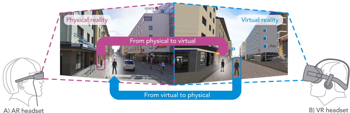
Fig. 2. AR and VR based telexistence system allows different located users be present in same place in different realities through AR glasses (A) VR headset (B).
