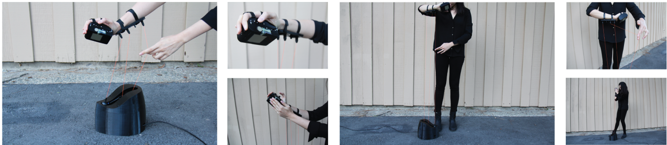
Figure 1: Bodyharp consists of two wearable interfaces (attachment to the performer's arm and a hand controller) and a main instrument body.
