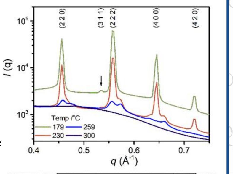
Disordering of the structure results in partial collapse of the pore structure.
