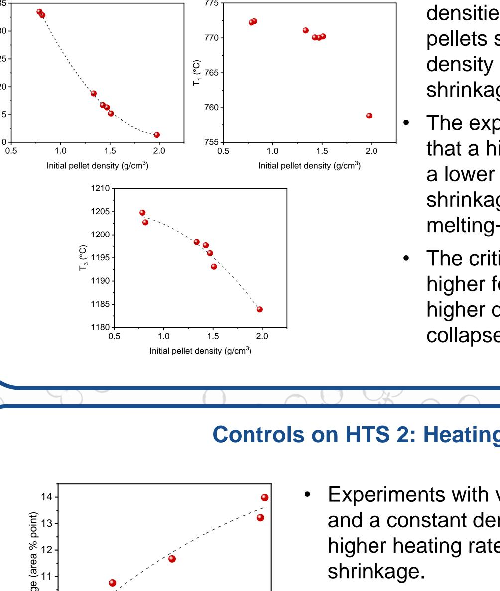
densities of the stone wool pellets show that higher density results in less shrinkage
