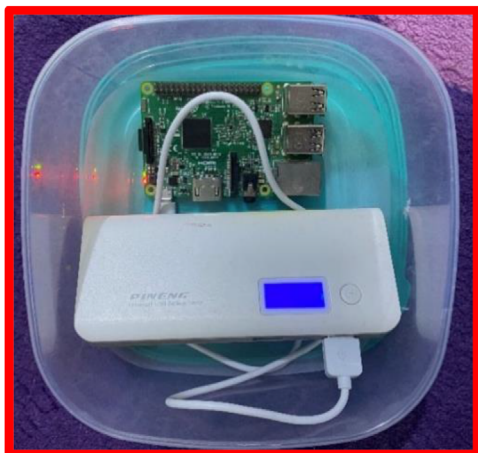
FIGURE 8 Structure of base station unit
