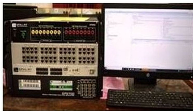
FIGURE 15 Experimental setup based on OPAL-RT
