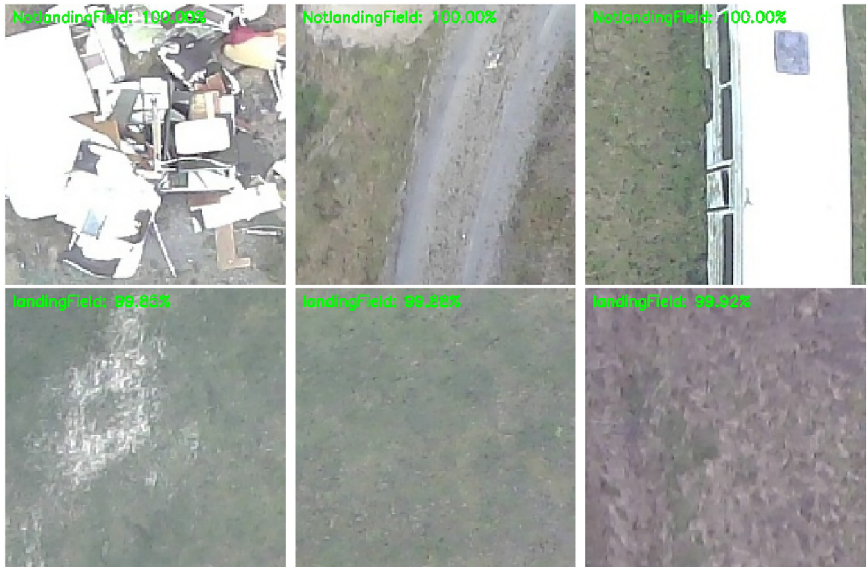
Figure 13. Results from the keras classifier after the dropout layer is applied. Top text shows whether the frame can be considered, and the percentage of confidence in the classification.
