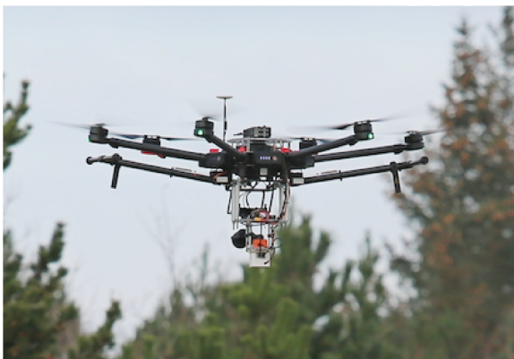
Figure 2. SafeEYE lab is mounted on a DJI M600 drone. The white box at the bottom is SafeEYE lab, with an extra IMU on top (orange). Behind SafeEYE lab is a standard X5 camera. The payload radio is mounted on the top of the aircraft. The image is from Oksbøl on December 4, 2019.
