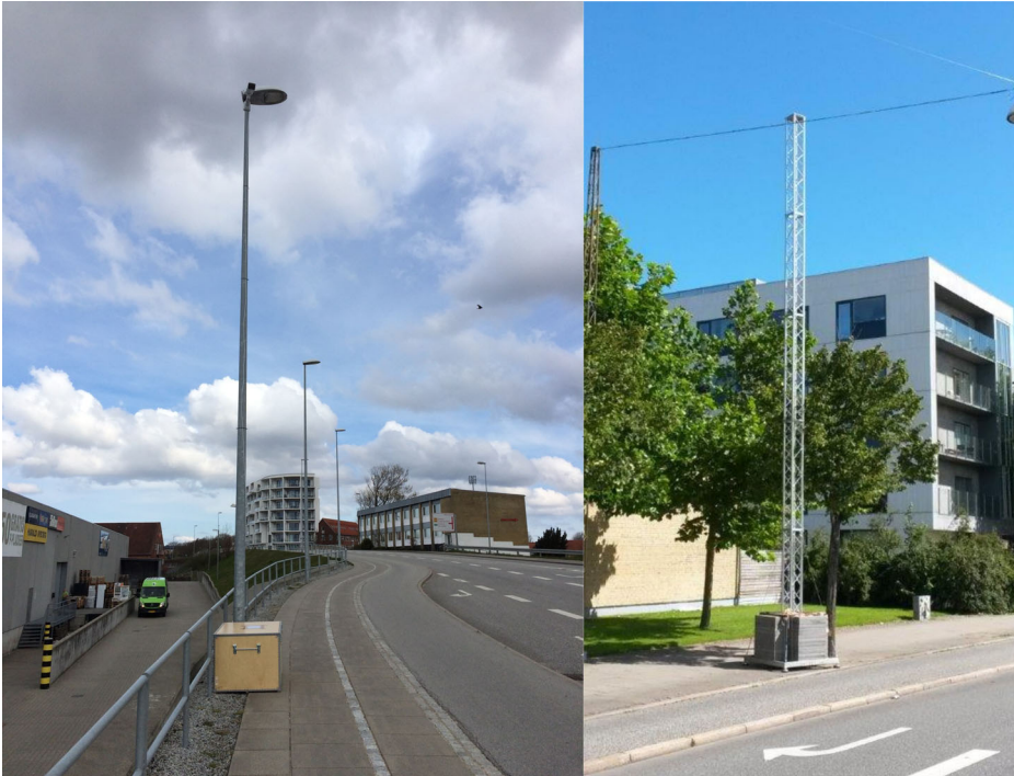
Figure 4. Camera setup for collection of video footage. Existing lighting poles were used where possible (left). Alternatively, a mobile pole (right, sites 3, 4, 6 and 7) was used to ensure a good camera position.
