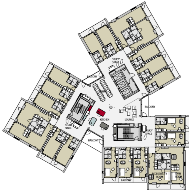
Figure 4. Horizontal social spaces. Floor plan of the Campus College’s sixth floor. At Campus College, every floor has a shared kitchen and living room located in the distribution area next to the elevator in the core of the three residential areas with a total of 21 units. Source: Mechlenborg and Hauxner (2021, p. 45), with the courtesy of C. F. Møller Architects.
