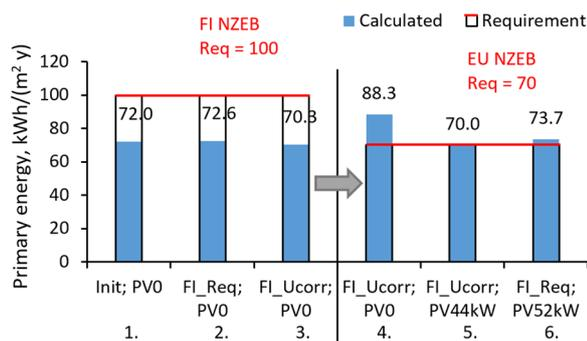
**Fig. 6.** Annual PE consumption of the reference office building. Finnish cases calculated according to Finnish methodology (cases 1-3) and EU standardized methodology (cases 4-6), all cases with Finnish TRY. [Code: *Init* – Initial building parameters; *FI\_Ucorr* – Finnish climate-corrected U-values; *FI\_Req* – Finnish minimum requirements for U-values; *PV\_44* – accounting for 44 kW of PV-panels].
