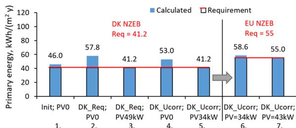
**Fig. 5.** Annual PE consumption of the reference office building. Danish cases calculated according to Danish methodology (cases 1-5) and EU standardized methodology (cases 6-7), all cases with Danish TRY. [Code: *Init* – Initial building parameters; *DK\_Ucorr* – Danish climate-corrected U-values; *DK\_Req* – Danish minimum requirements for U-values; *PV\_49* – accounting for 49 kW of PV-panels].
