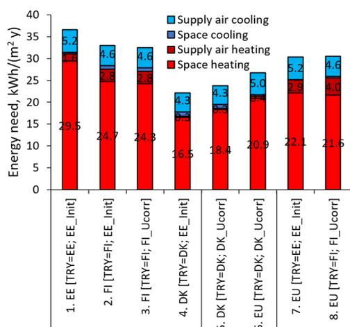
**Fig. 3.** Comparison of annual energy need (net energy) for heating and cooling using country specific climate data, methodologies, and climate corrected U-values. Calculated according to Estonian (EE), Finnish, (FI) and EU standardized (EU) methodology and input data.
