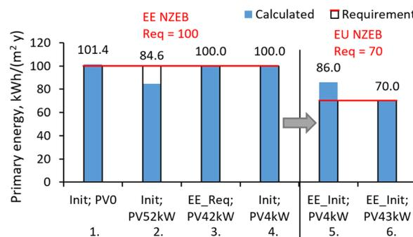
**Fig. 4.** Annual PE consumption of the reference office building. Estonian cases calculated according to Estonian methodology (cases 1-4) and EU standardized methodology (cases 5-6), all cases with Estonian TRY. [Code: *Init* – Initial building parameters; *EE\_Req* – reduced requirements for U-values; *PV\_42* – accounting for 42 kW of PV-panels].
