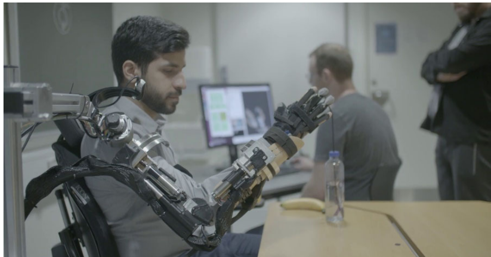
Figure 2. The EXOTIC exoskeleton system. An individual commands the EXOTIC exoskeleton using a tongue interface shared with computer vision-based semi-automation. The individual shown in the image has given written consent to the use of the image.
