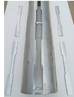
Fig. 6 Specimens for tensile test cut from tube along longitudinal direction.
