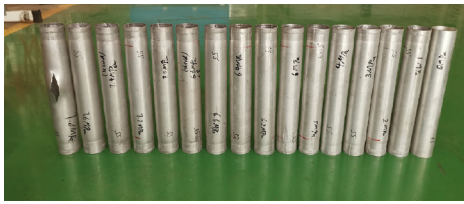
Fig. 9 Tubular specimens before and after hydraulic test.
