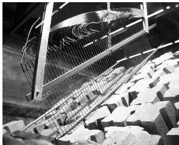
Figure 3: A novel step gauge for laboratory wave run-up measurements on a breakwater slope (designed and constructed at Ghent University).
