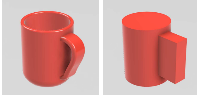
Figure 13. Example of an object and its decomposition into primitive shapes. This approach was used by Milleret et al. [39].
