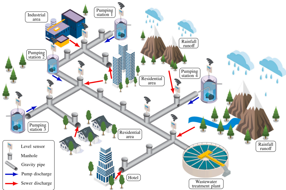
Fig. 1. An illustration of a pumped wastewater network, where water level sensors are deployed in critical points.
