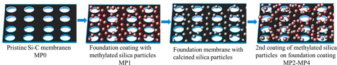
**Fig. 1.** A schematic diagram of the Si-C membrane modification via foundation particle coating, calcination and surface particle coating. Silica particles and methylated silica particles are illustrated with simple spheres and spheres with the circle around, respectively.
