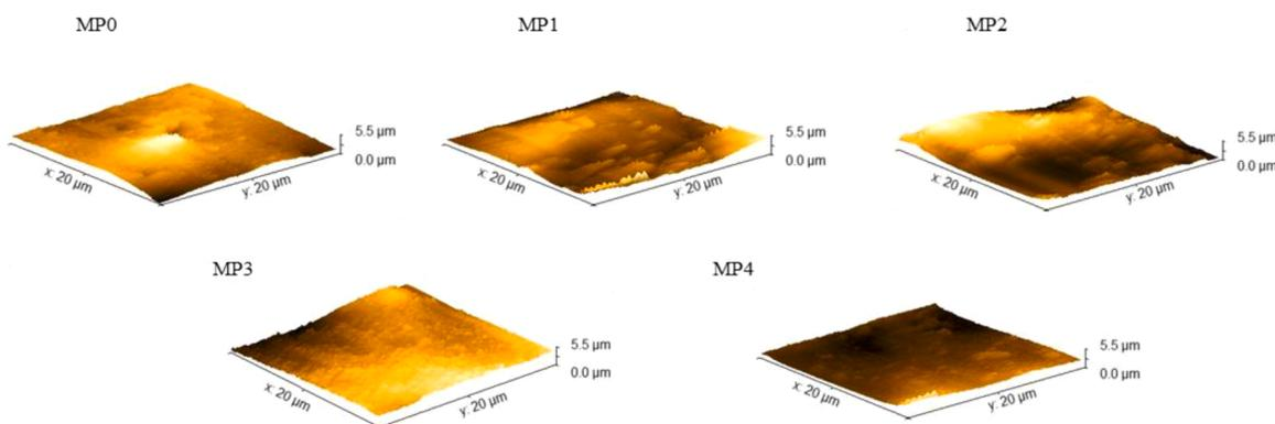
Fig. 6. AFM images of the membrane surfaces.
