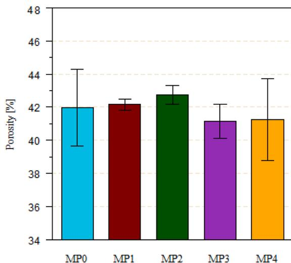
Fig. 7. Porosity of the pristine and modified membranes.
