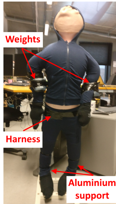
Figure 2. View of the created low-cost doll, together with clothes and ankle weights.
