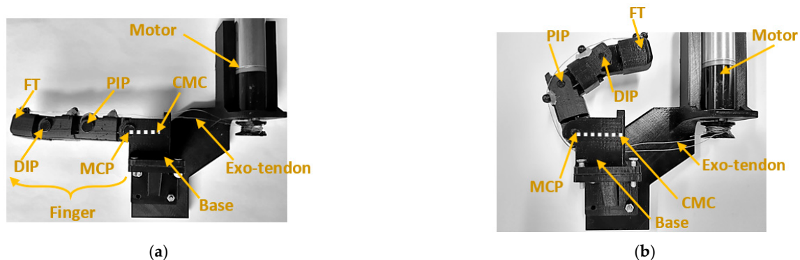
Figure 5. Artificial finger in its initial position for assessing (a) flexion and (b) extension. Note: the exotendons are not under tension since the artificial finger is in a relaxed state.
