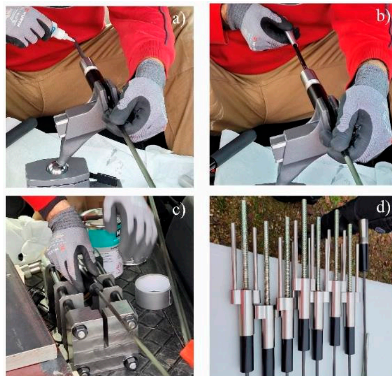
Figure 7. Assembling of the CFRP anchors. Photographs by the authors. (a) Grinding the CFRP surface and lubricating the surface with thin, liquid, and fast-curing glue. (b) Mounting of the wedge (viii) on the 8 mm CFRP rod in the lubricated area, which is then assembled with the barrel (ix). (c) Pre-setting of the wedge into the barrel using approximately 120 kN. (d) The coupler with inner threads (vii) was assembled with the threaded bar (v) as well as the end-threaded counteracting torque pins (vi) and screwed onto the threaded barrel (ix). Photographs by S&P.
