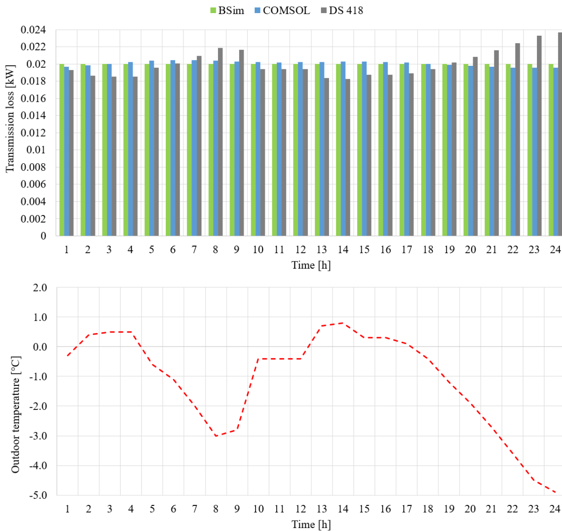
Figure 14. The transmission loss for the 1 st of January using the construction element equipped with 300 mm wood fiber insulation.
