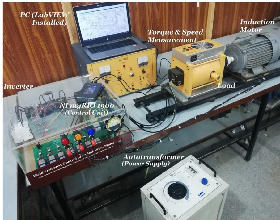
FIGURE 4 Induction machine drive testbed set-up
