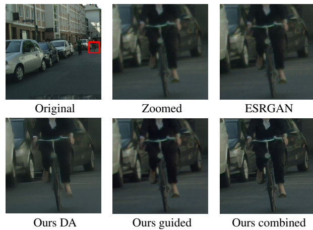
Figure 1: Super-resolution ( \times 4 ) of a real image from the Cityscapes dataset [11]. By combining domain adaptation (DA) and guidance by semantic segmentation, our proposed method reconstructs visually pleasing images. In contrast, ESRGAN fails to handle the corruptions in the real image, resulting in many artifacts.
