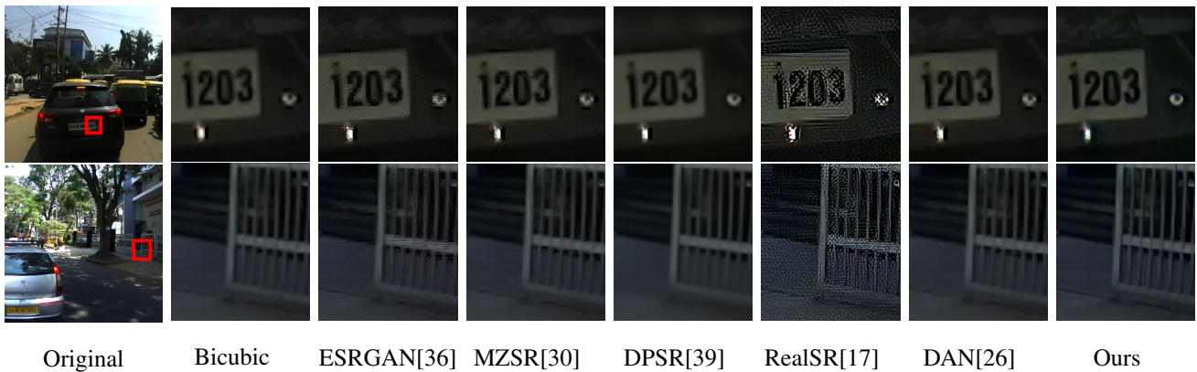
Figure 5: Comparison with SoTA methods for \times 4 SR of real images from the IDD dataset. As visible, our method reconstructs more detailed images with less artifacts compared to the existing methods.
