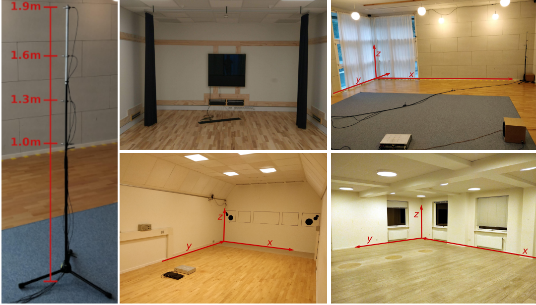
FIG. 1. Left: Rig with four microphones. Rooms from top left to bottom right: Room B, VR Lab, Listening Room, and Product Room.
