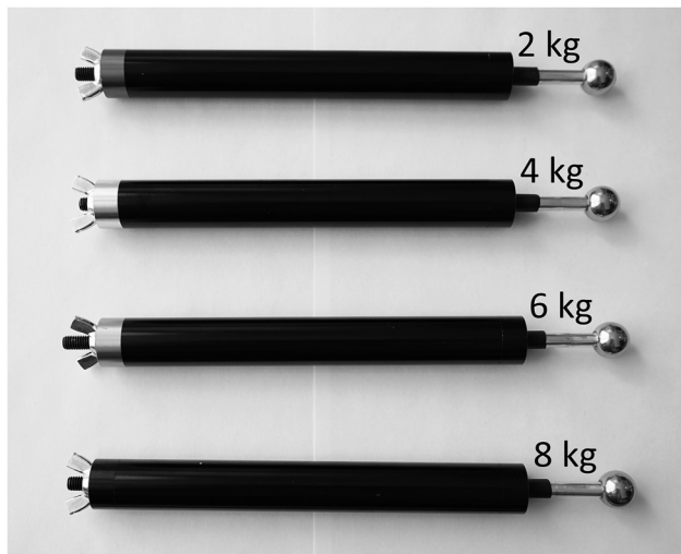
Figure 1: The four probes utilised in the present study with the respective calibrated pressure. The probes are approximately 0.23 m long. Developed and calibrated by University of Southern Denmark, Odense, Denmark.
