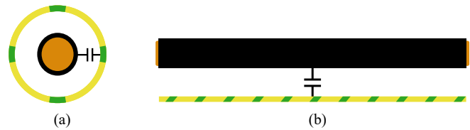
Fig. 21. Cable common-mode capacitive couplings for a) a shielded cable and b) a cable in close proximity to a grounded surface.
