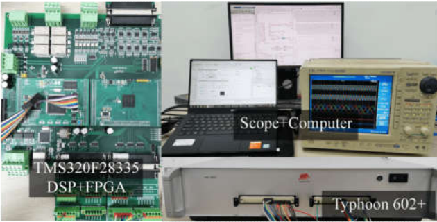
Fig. 16. Hardware platform of CHIL experiment.
