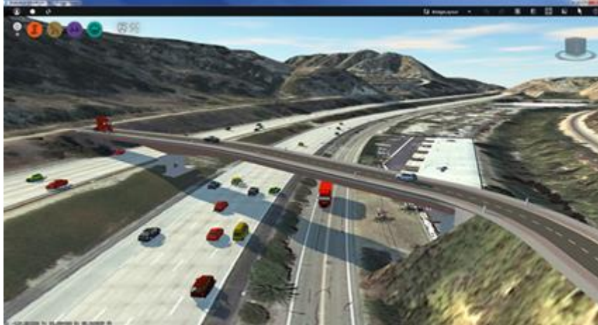
Figure 6.13 Infrastructure networks modelled as 2D cut-through sections that are swept along paths.
