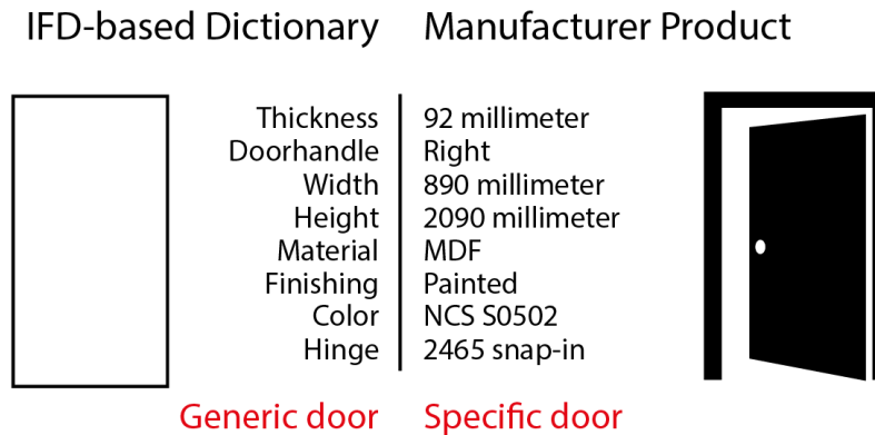
Figure 4.12 Definition of a generic door, represented using the IFD standard (left), and the way in which it is used in the definition of a specific product (right) 21 .
