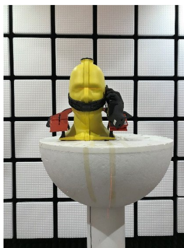
Figure 2: Voice mode with phone next to the left-hand side of the head phantom placed in A left-hand phantom (beside head hand left – BHHL).
