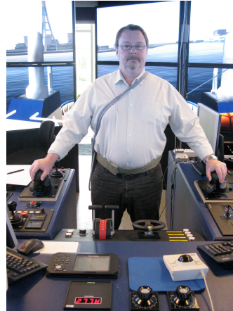
Figure 1. Simulation setup with tugboat pilot using a tactile belt
