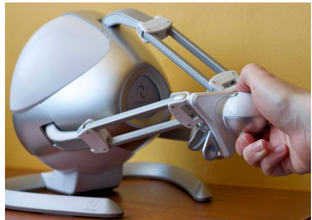
Figure 3. A picture of the NOVINT Falcon force feedback device used to allow haptic interaction with the environment.
