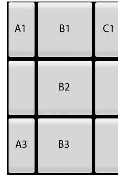
FIGURE 2. The button layout on the touch screen. B1, B2 and B3 are used to select the scanning distance, A1 selects guiding mode, C1 scanning mode, and A3 the POI to be guided to.
