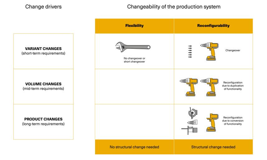
**Figure 2.4.** *Different levels of changeability for variant, volume, and product changes.*
