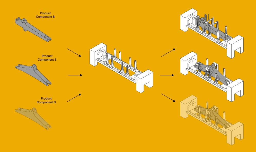
Figure 10.3. Illustration of modular and reconfigurable welding fixtures.
