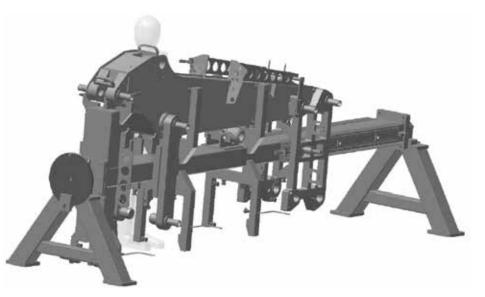
Figure 10.2. Illustration of one of the many dedicated welding fixtures.
