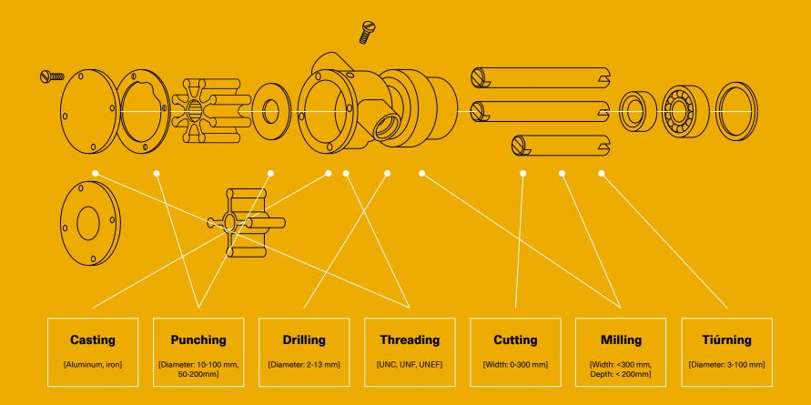
**Figure 7.2.** An example of how components in a product relate to production process capabilities.
