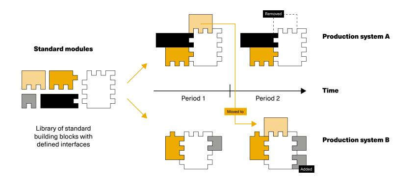
**Figure 3.2.** *Standard modules allow for different configurations in a production system.*
