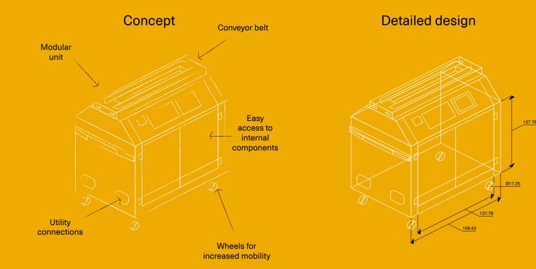
Figure 8.2. From concept to detailed design.
