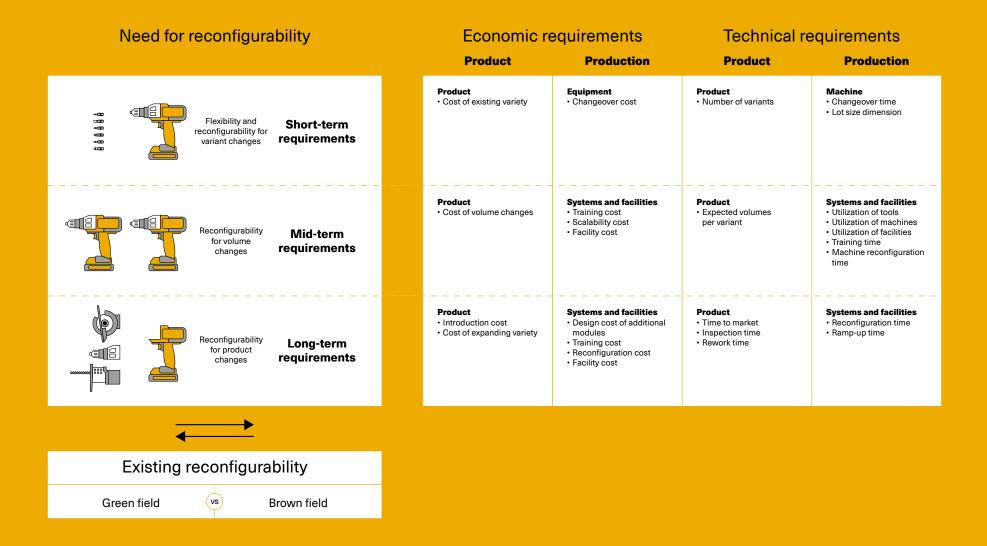
**Figure 6.4.** *Examples of economic and technical requirements in relation to the need for reconfigurability of production.*
