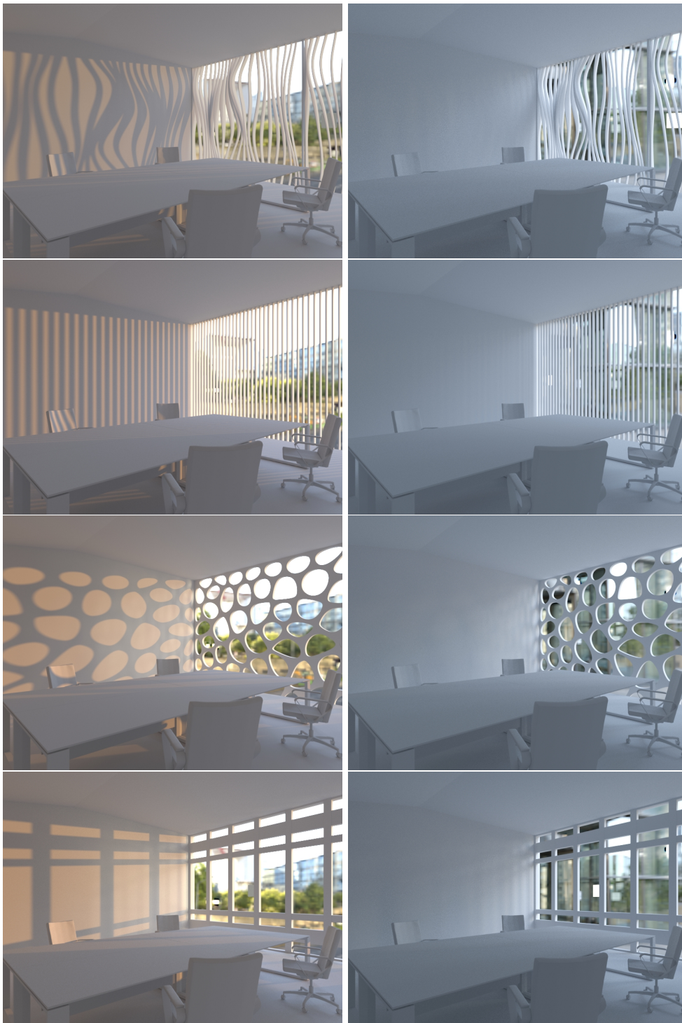
Figure 9. From top to bottom. A: Deformed Vertical Strips, B: Vertical Strips, C: Voronoi Tessellation, D: Regular Openings. All rooms were simulated under two different lighting conditions, direct sunlight and overcast.
