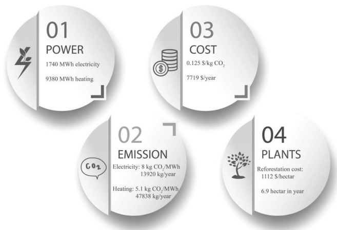
Fig. 19. Techno-economic-environmental benefits of the proposed smart system for a neighborhood with 100 building complexes.
