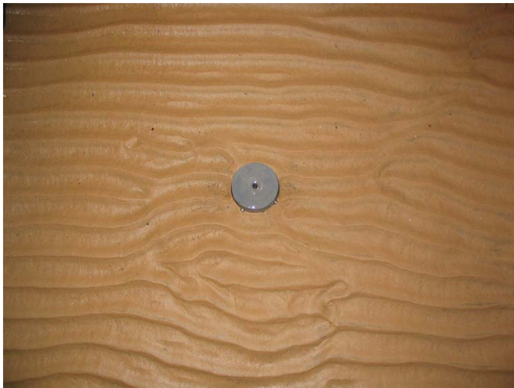
Figure14. The picture is from test 1.1. In tests 1.1 – 1.4 and 3.1 – 3.3 the scour depths are mainly caused by ripples.
