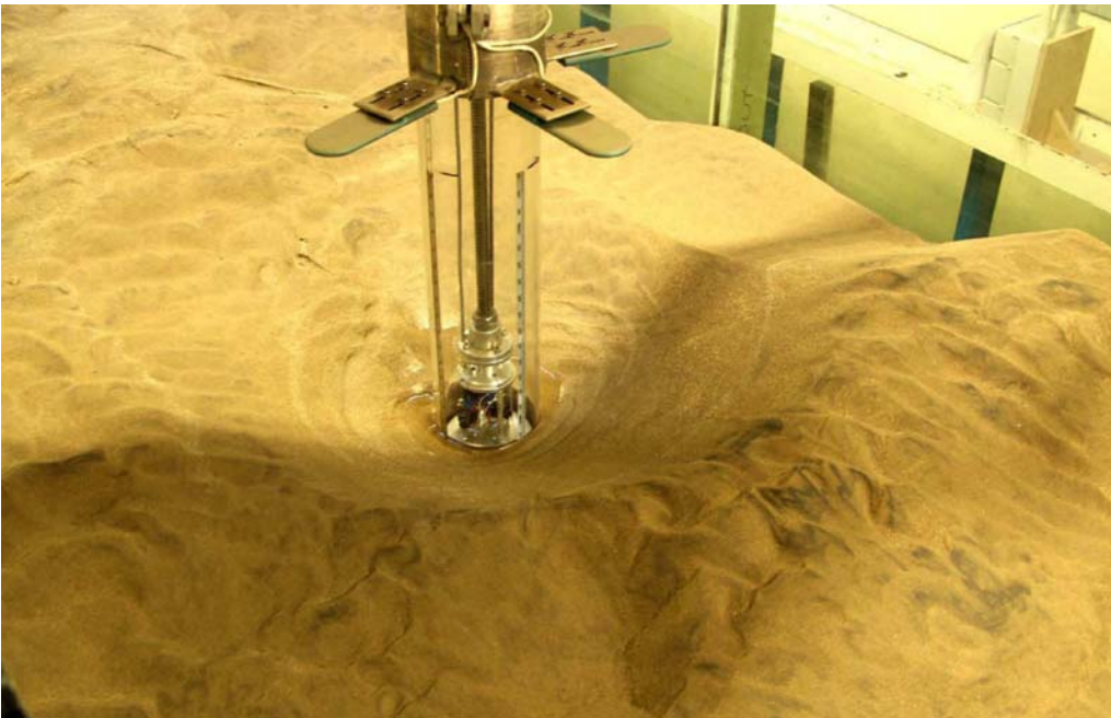
Figure 5-6: A live-bed scour hole.
