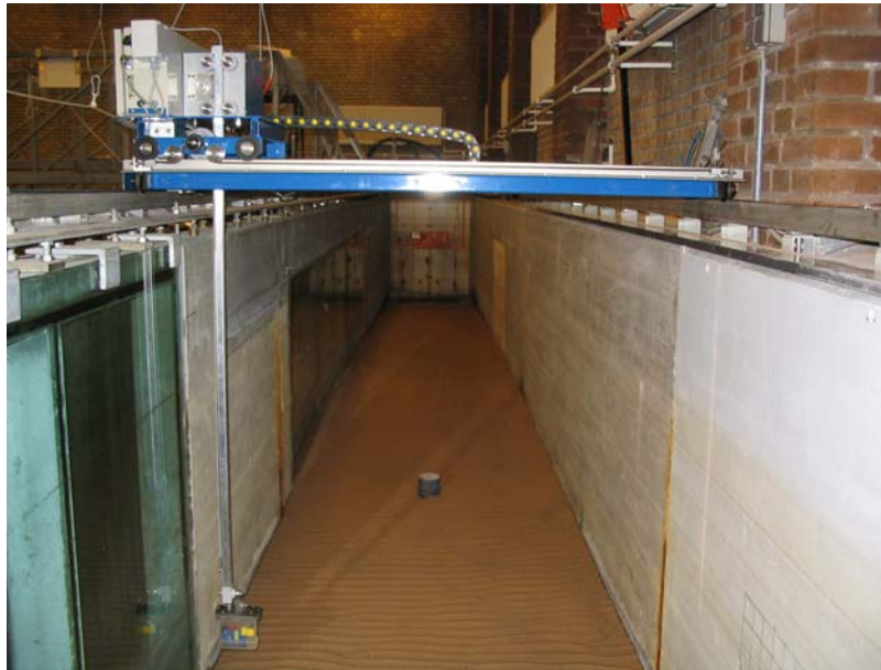
Figure 11. The bed has been measured with a profiler. A laser measuring the bed level in a grid.
