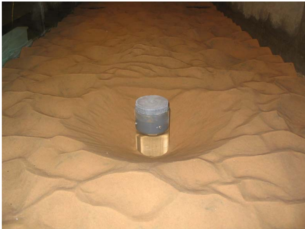
Figure 16. The picture is from test 2.2. In tests 2.1 – 2.9 the local scour holes around the pile are of significant magnitude in comparison to the ripples and the global scour.
