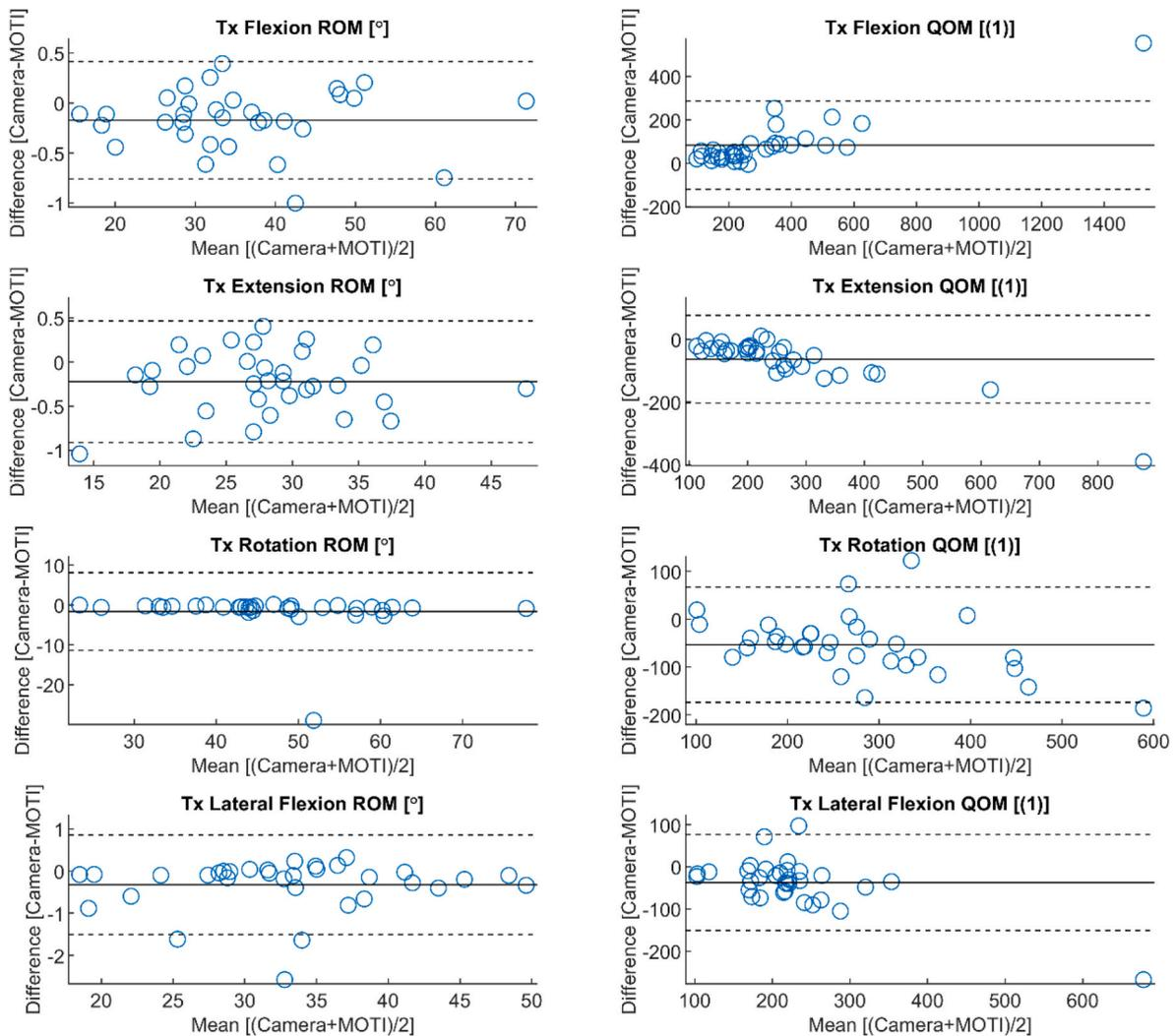
**Fig. 5.** Bland-Altman plots for trunk/thoracic (Tx) movements: ROM and QOM. The continuous line represents the mean of differences, and the dotted lines represent the limits of agreement. ROM was measured in degrees [°] and QOM is unitless [(1)].
