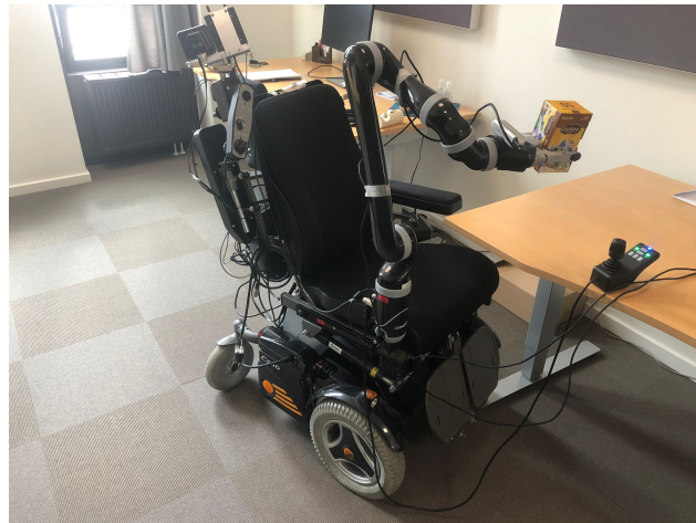
Figure 1. The JACO 2 robot arm attached to a wheelchair. A RealSense D435 Red Green Blue-Depth (RGBd) camera is attached to the end effector, which is holding a tea carton. The robot arm is controlled semi-autonomously by the user via a tongue-computer-interface (TCI).
