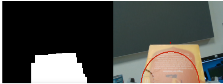
Figure 4. The resulting binary mask (left) and the original RGB image with the ellipse estimating its size (right). The ellipse results from fitting it to the largest boundary of the binary mask. For this specific setup, since the gripper is at the very bottom of the frame, the assumption can be made that the object is also always at the bottom. Hence, a half-dome shape was used by point rotation of the mask by 180° and fitting the ellipse to it.
