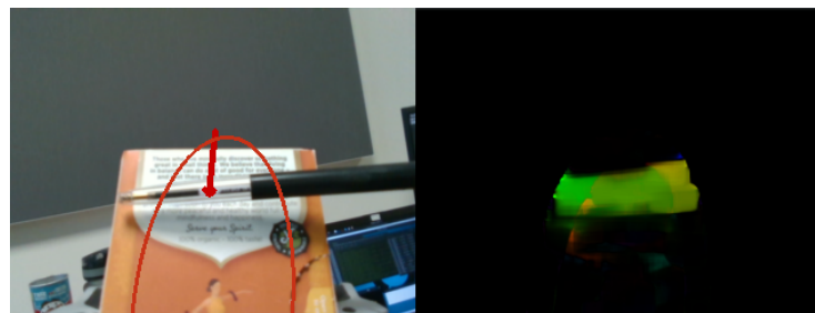
Figure 5. A pencil occluding the optical path of the camera to the object without causing slip to be detected. If an actual slip case would occur, more than 50% of the non-zero-magnitude pixel would show optical flow (OF) above the threshold, triggering slip to be detected even if the obstructing object is still.
