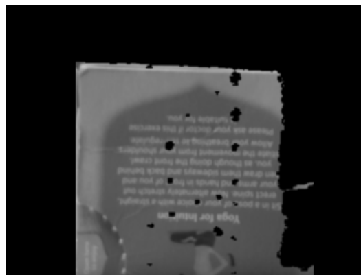
Figure 3. Example of a still noisy grayscale image of an object with the background mostly removed. Here, objects and movements close to the grasped object could cause the boundary of the objects to extend and include some of the background in the boundary estimation.
