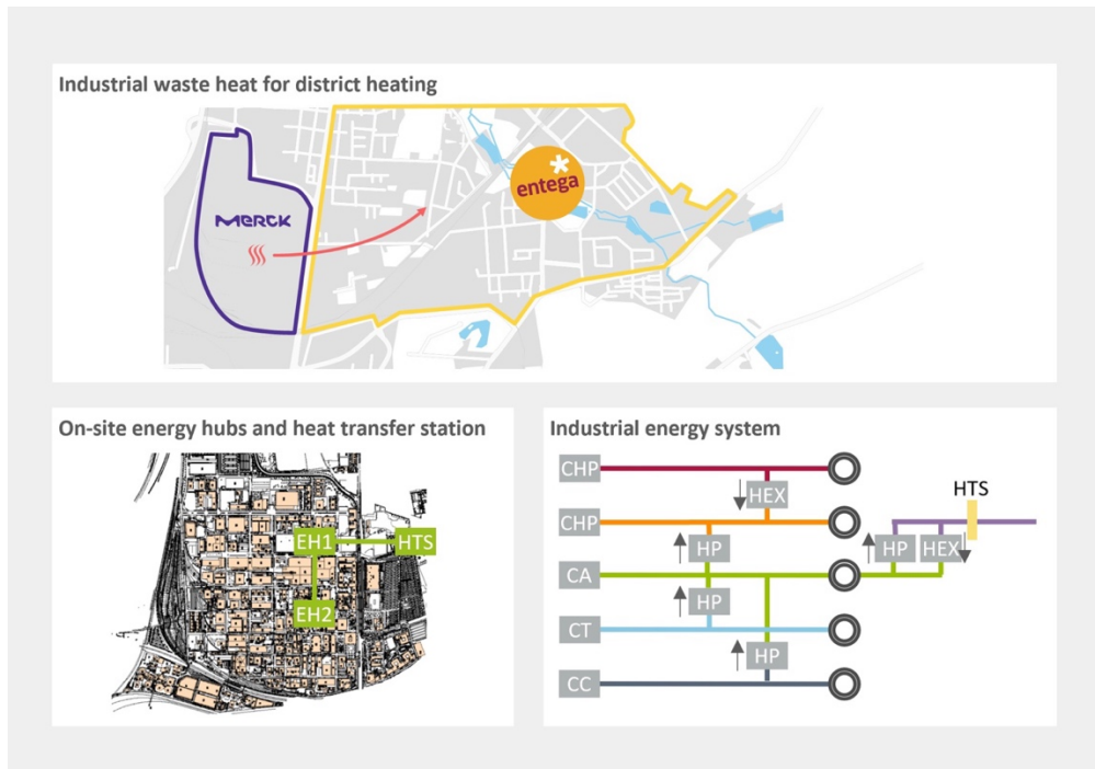
Figure caption: Interacting energy-optimized industrial district (EH: Energy hub, HTS: Heat transfer station, CHP: Combined heat and power, CA: Compressors for pressurized air, CT: Cooling tower, CC: Compression chiller, HEX: Heat exchanger, HP: Heat pump, colored lines: heating and cooling networks on different temperature levels)
