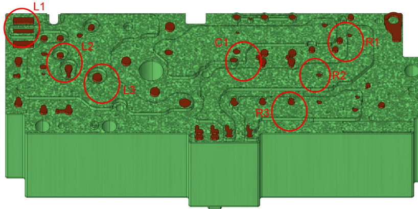
Fig. 6. Numerical model of the PCBA under test with pinholes created on the solder mask (backside view).
