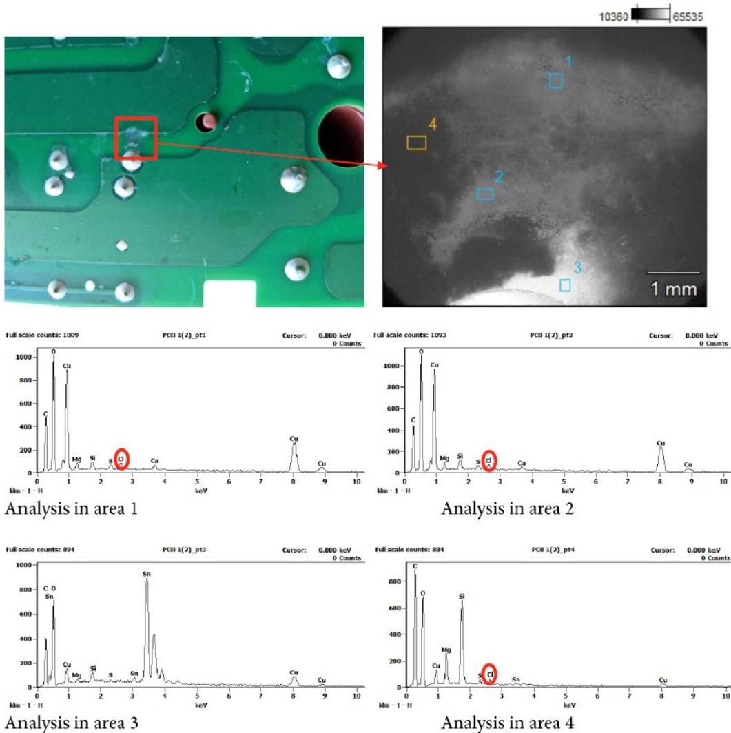
Fig. 2. FE-SEM analysis of the PCBA under test.
