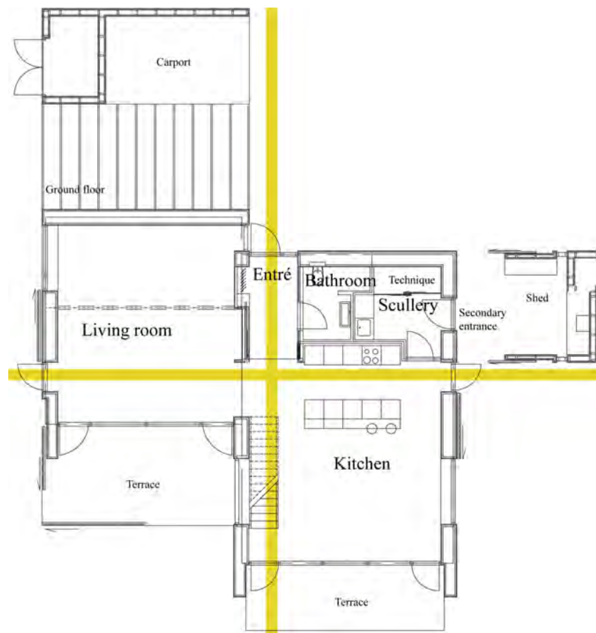
Fig. 4. Plan drawing of the ground floor illustrating the entrance from the north, the living room facing south-west and the central kitchen dining room facing south. The yellow "light cross" illustrates the light openings in all four directions.
