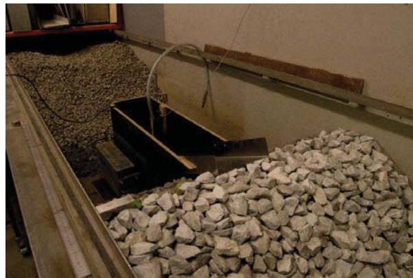
Figure 1: Set-up of overtopping tank.
