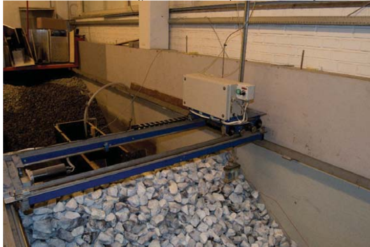
225 Figure 8. Profiler used to measure the eroded area.
