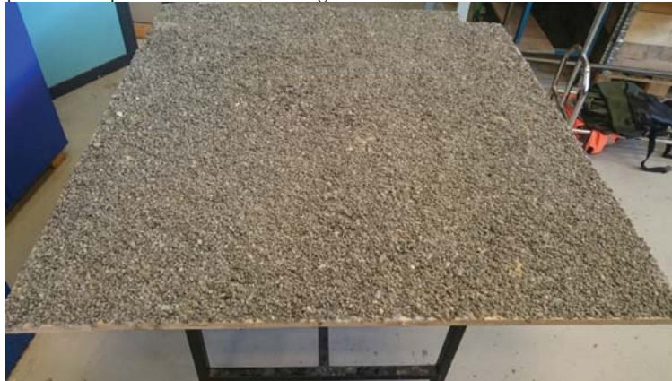
165 Figure 5. Plywood plate with glued Class V rocks. Used to increase the roughness of the impermeable 166 interface.
