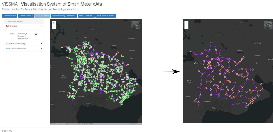
Fig. D.3: Overview of the WebGIS application and its features. The medium-voltage part of the visualization includes secondary substations and their interconnections
