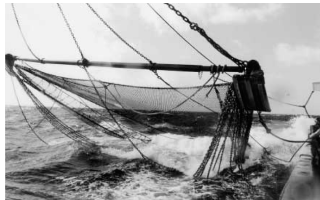
Beam trawl: One of the most fuel consuming fishing practices, which also affects the seafloor.
