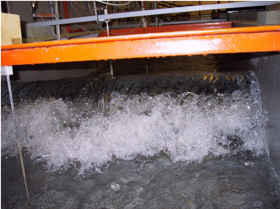
Figure 23: Breaking of a wave propagating the steep reef-slope during the tests.
